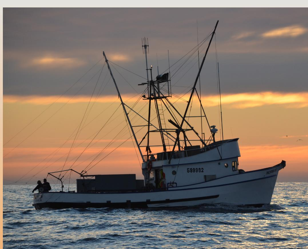
Oregon albacore are caught one at a time using fishing lines attached to outriggers that extend out from the sides of the boat. Tuna is also caught using bait on individual poles. These types of fishing, sometimes called trolling, prevent the accidental catch of other animals (called by-catch) such as sea turtles and dolphins.
